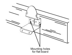
To mount the bracket on a round post, use the inner holes.
