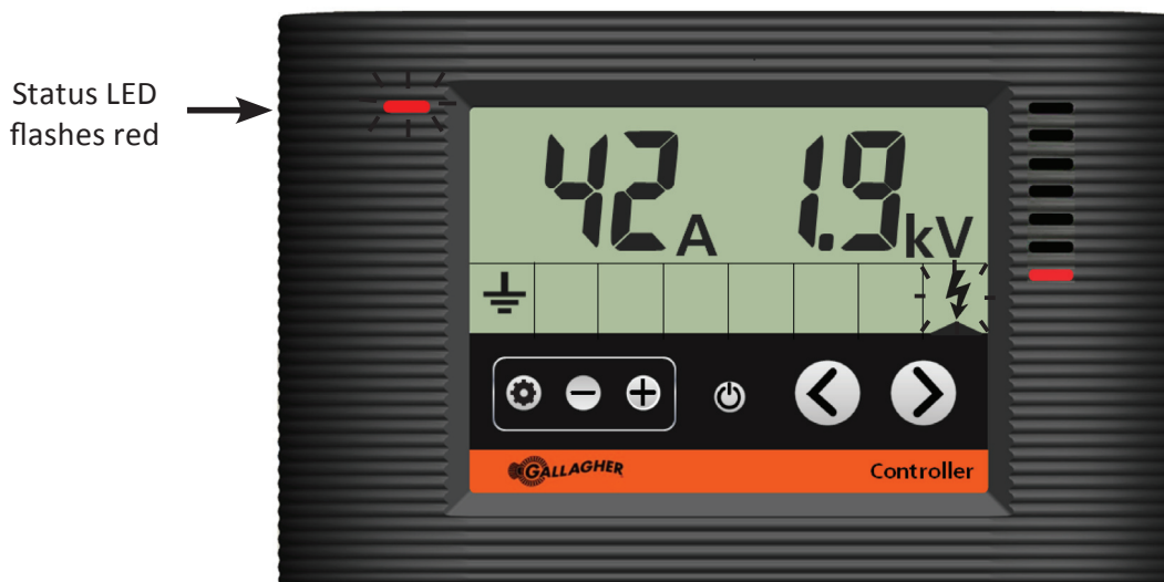
Controller showing the energizer in current alarm
