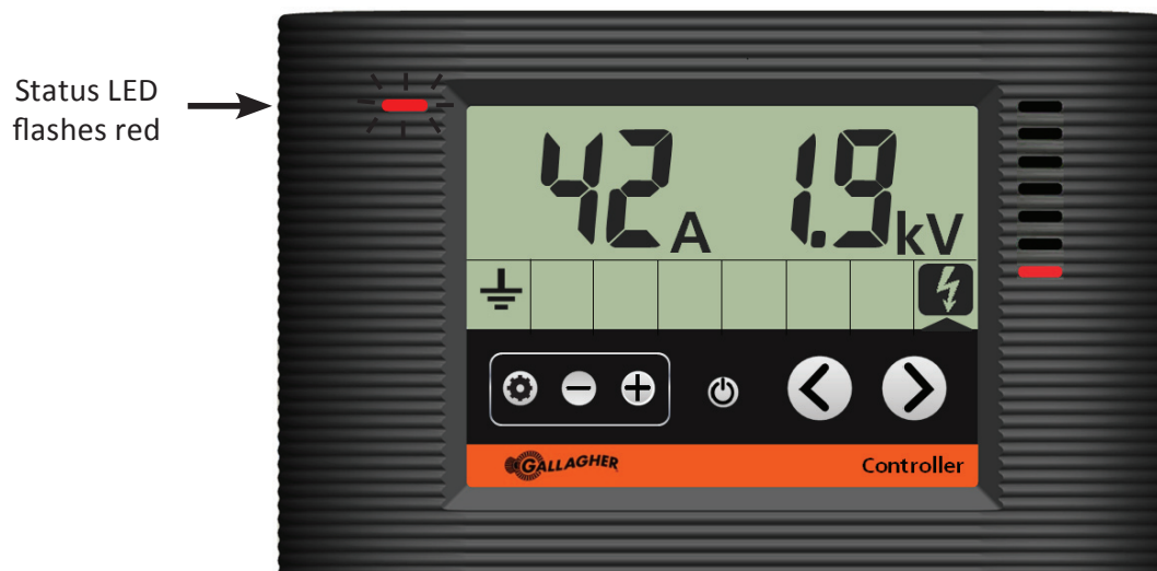
Controller showing the energizer in output alarm
