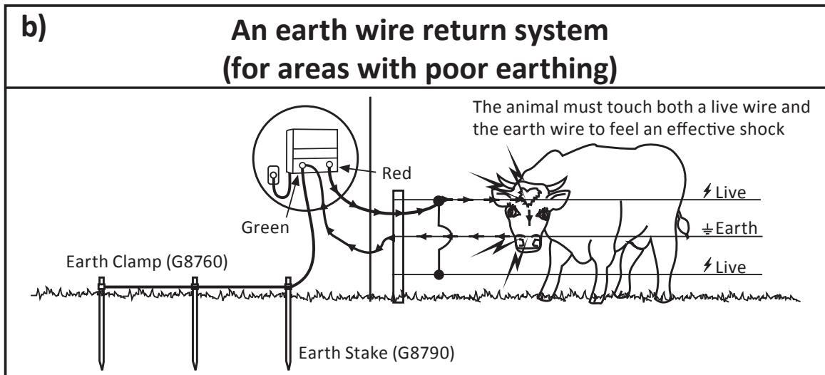
Earth stakes, at least 2m (6ft) long, should be spaced 3m (10ft) apart. Use a minimum of 3 earth stakes for the M150, M300, M500.
