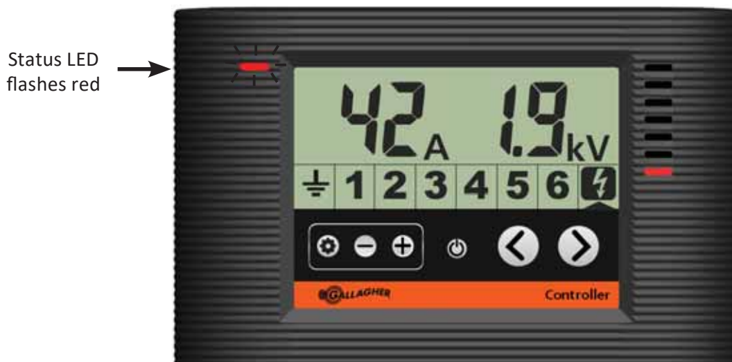
Controller showing the energizer in output alarm
