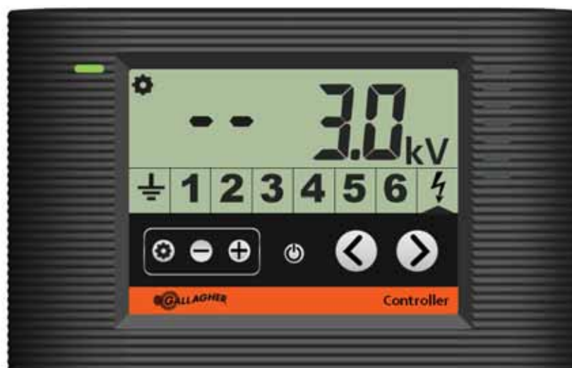
Controller showing the default energizer alarm setup with current disabled and voltage at 3.0KV
