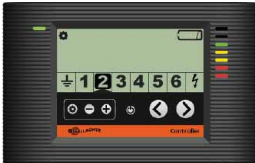
Controller showing zone 2 with a low battery
