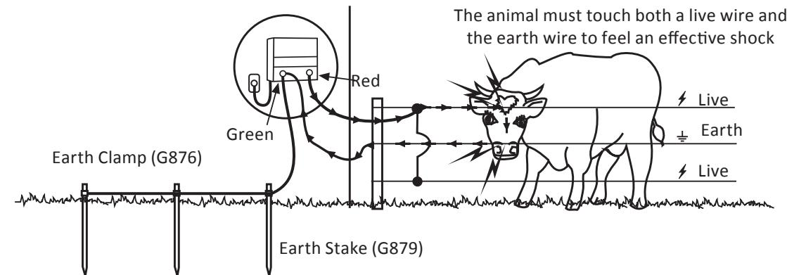
Earth stakes, at least 2m (6ft) long, should be spaced 3m (10ft) apart. Use a minimum of 3 earth stakes for the M1000.
