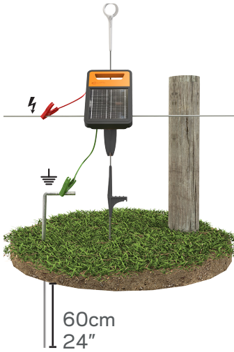
Earthing for Step 3 (a. b. c.)
