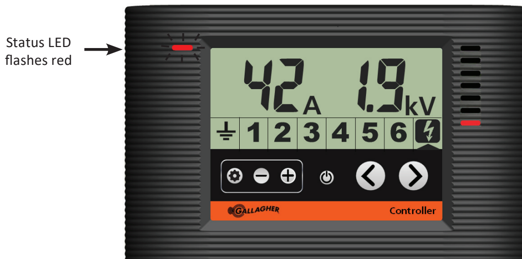
Controller showing the energizer in output alarm
