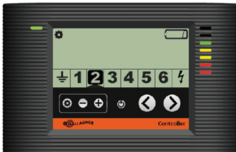
Bedieningspaneel toont zone 2 met lege batterijen
