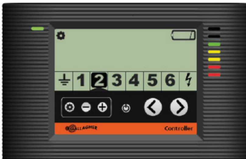
Controller showing zone 2 with a low battery
