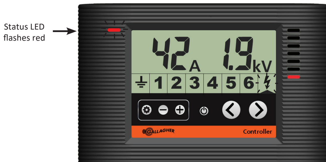
Controller showing the energizer in current alarm
